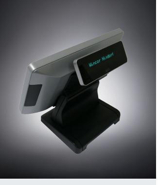
**BA64-G** is equipped with a LCD graphical display that allows for up to 4 rows at 30 characters of 8x16 pixels. Complex characters like Asian or Arabic can be shown in a 2-line mode.
